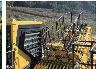
Boom catwalk with handrails
