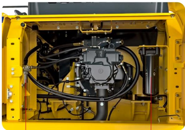
Pilot filter (Attachment piping specification)
