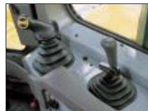
PPC control combined with the highly reliable Komatsu hydraulic system enables superb fine control. (Dual tilt and pitch operation are enabled by depressing switch with a thumb. This is available when optional dual tilt dozer is installed.)
