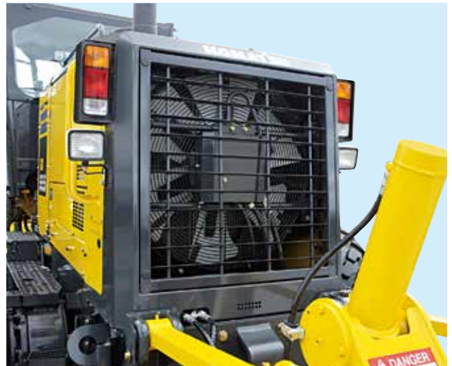
Hydraulic driven cooling fan
