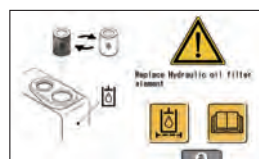
Clogging hydraulic oil filter caution
