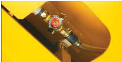
Fuel drain valve
