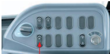
Dual mode engine power selection switch
